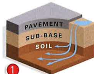
2 The moisture freezes when temperatures drop, causing the ground to expand and push the pavement up.
