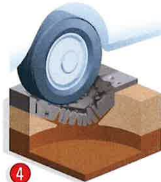
2 The moisture freezes when temperatures drop, causing the ground to expand and push the pavement up.
